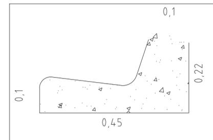
DETALHE DA GUIA E SARJETA S / ESCALA
